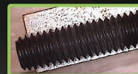
After 50x torquing Cleaning Grade 2
