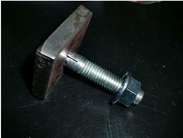
Figure 2.3 Complete tension test; pull-through
